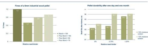
FlourBond<sup>®</sup> improves the pellet hardness by up to 15%. The optimal dosage of Flour Bond is between 0.5 and 2.0%. A higher addition has no further effects on the hardness of the pellets.
